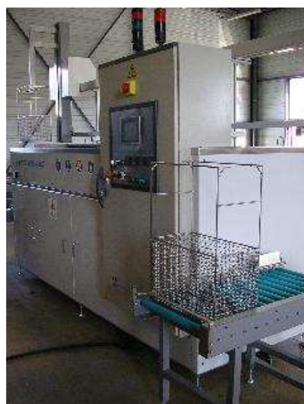
U2HF60 machine with robot and load/unload conveyors
